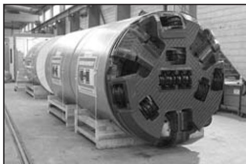
Microtunnel Boring Machine
