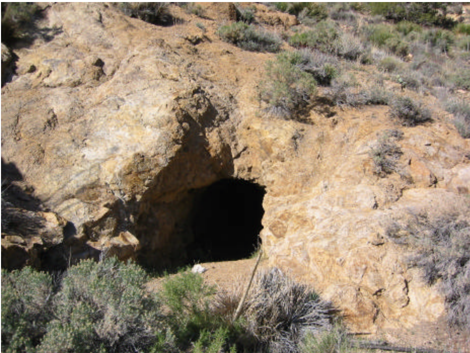
101-0165_IMG: A small mine adit (this adit extended only ~5 m into the hillside)
