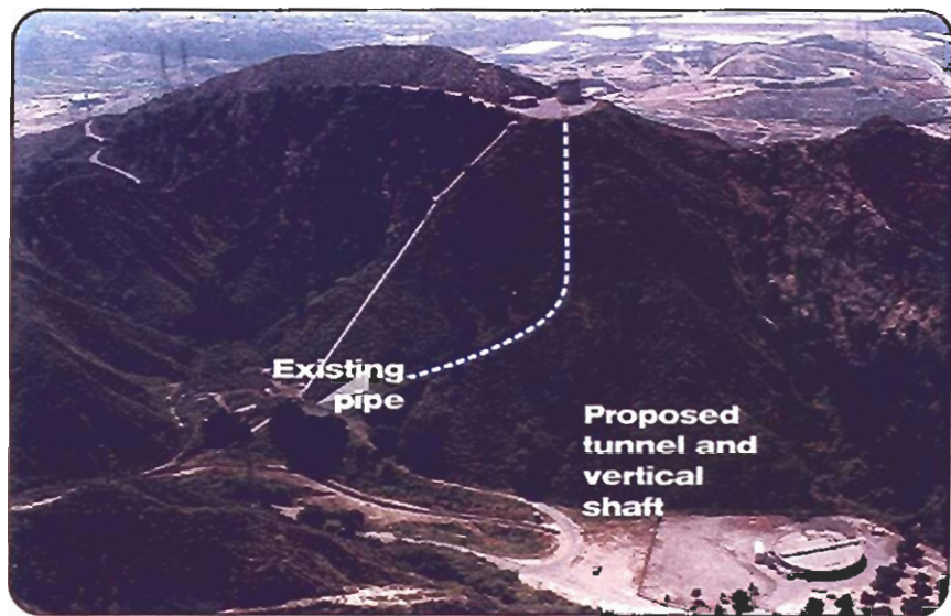
Existing Terminal Hill pipe and proposed tunnel.
