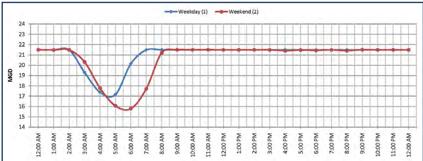
Figure 3-6: LAG Diurnal Dry Weather Influent Flows
