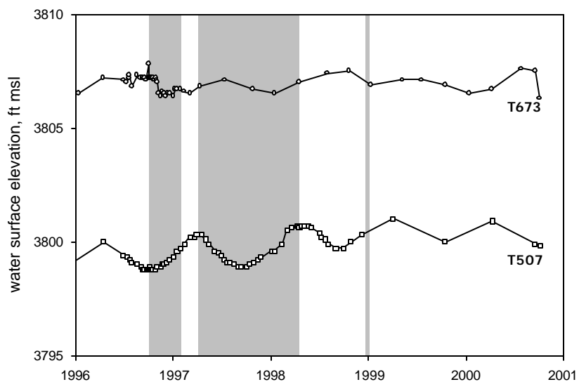
Figure 28. Shallow wells near 380W and 381W. Gray indicates when wells were on.
