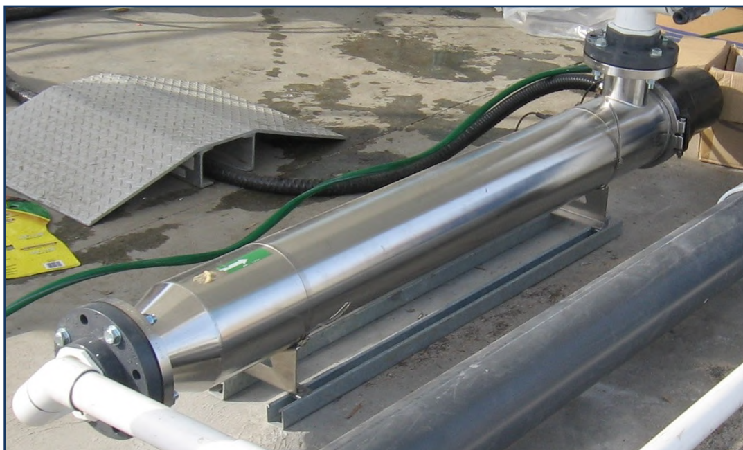
Figure 2-6: Pilot Testing UV Reactor
