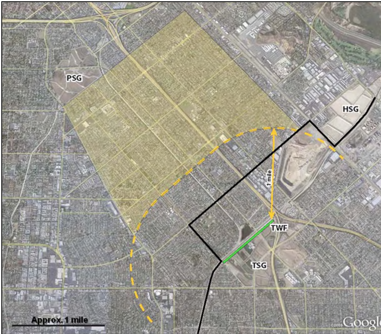
Figure 3-12: Potential Zone for Injection Wells
