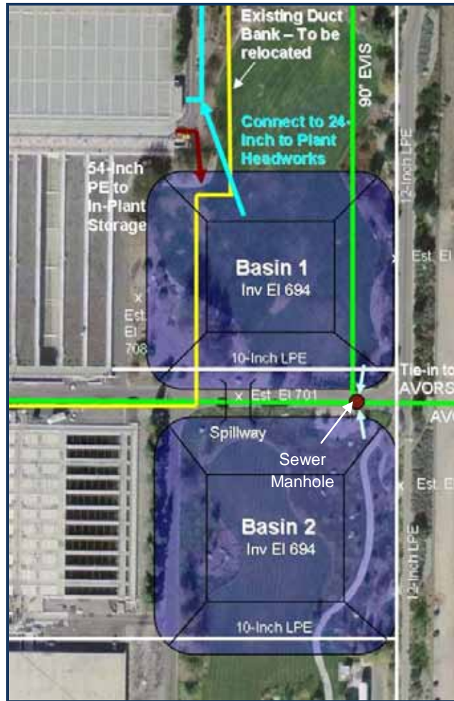
Figure 6-1: Location of Wet Weather Storage Basins
