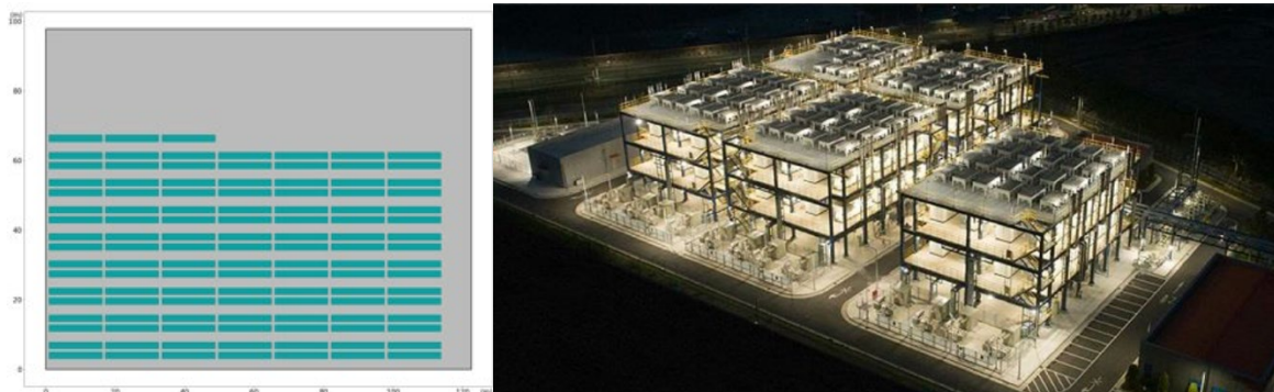
Figure C-1. Example of fuel cell layout in back-to-back rows (left). Example of a stacked layout in a city block type configuration (right).
