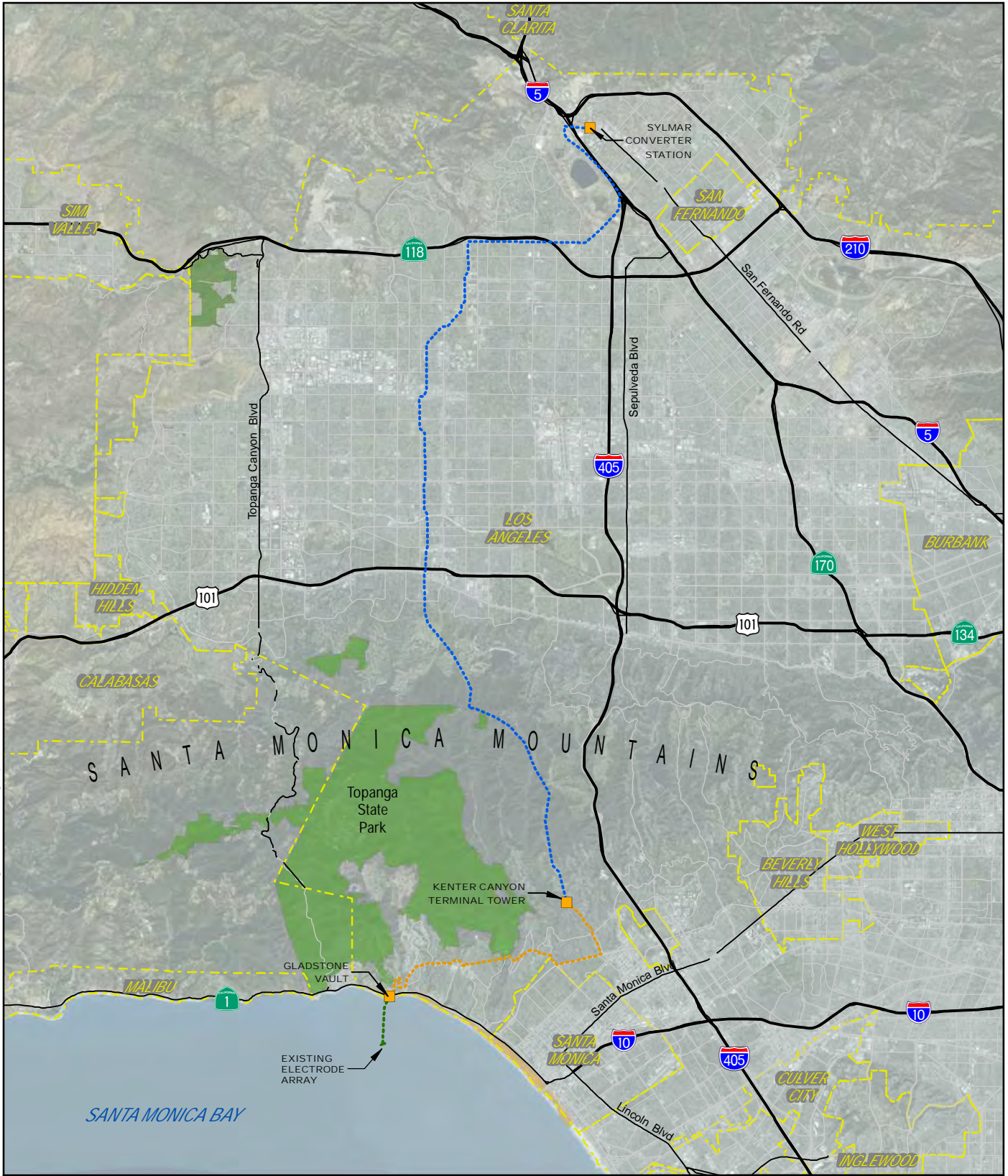
FIGURE 2-2 EXISTING SYLMAR GROUND RETURN SYSTEM
