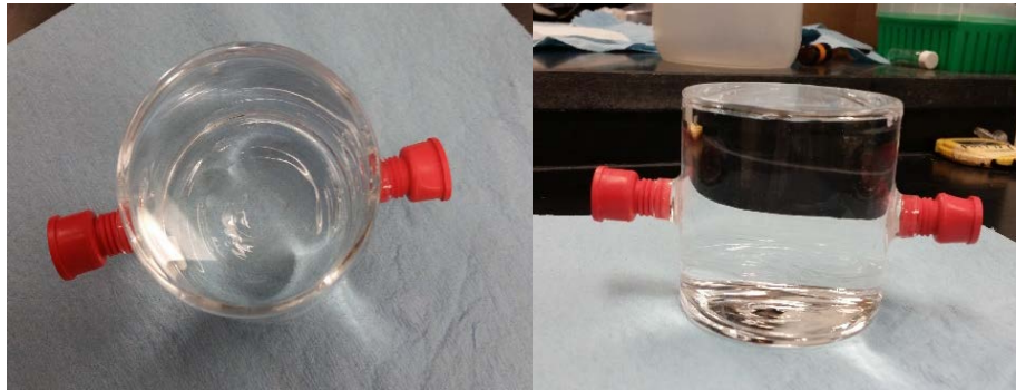
Figure 2-2. Quartz vessel used in the UV AOP analysis of VOCs and 1,4-Dioxane
