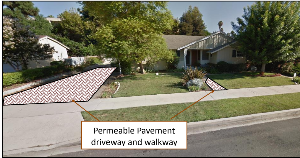
Figure: Example Plan View Configuration - Permeable Pavement Application on Single-Family Residential Property can include a Permeable Pavement Driveway and Walkway
