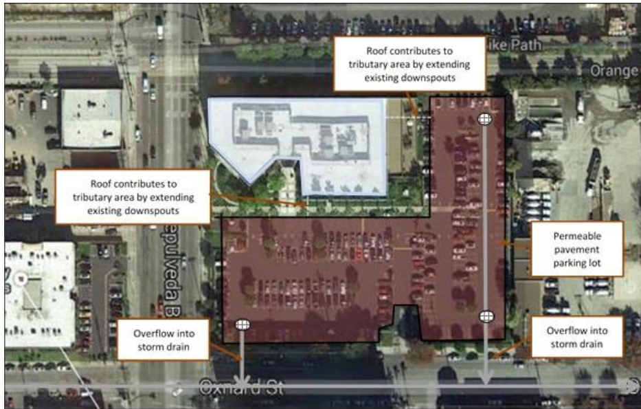
Figure: Permeable Pavement in a Church Parking Lot with Roof Runoff Contributing to Tributary Area
